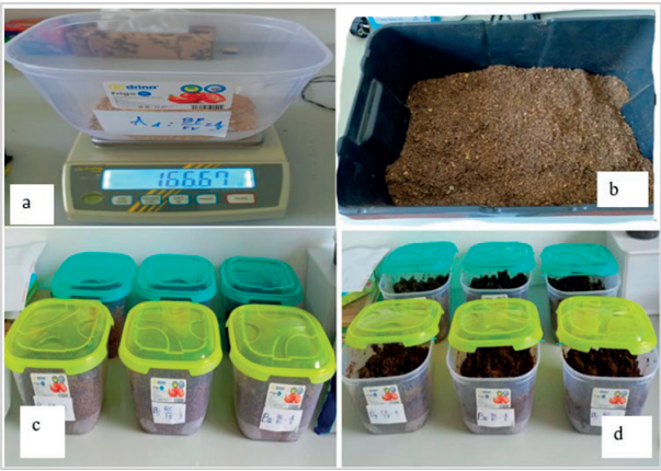
Photo 1. Stages preceding and during the composting process: weighing (a) and mixing of waste (b); filling of the composting boxes (c); phospho-composts during their evolution (d)
