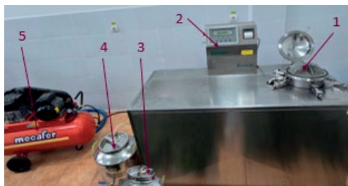
Figure 1. Timatic DUO percolator: 1 - extraction chamber; 2 - control panel; 3 - extract collection vessel; 4 - expansion vessel; 5 – compressor
