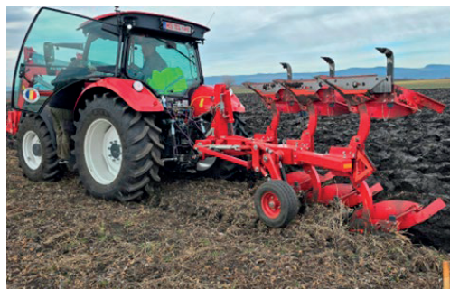
Figure 1. Application of basic soil tillage technology with reversible plough with bodies equipped with ploughshares, in the Dumbrăvioara experimental site (Mureș County)
