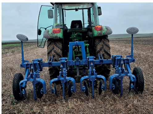
Figure 3. Application of technology with narrow strip tillage equipment, in the Dracea experimental site (Teleorman County)
