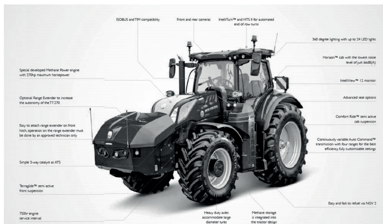
Figure 8. New Holland T7.270 Methane Power Tractor (Source: https://agriculture.newholland.com )
