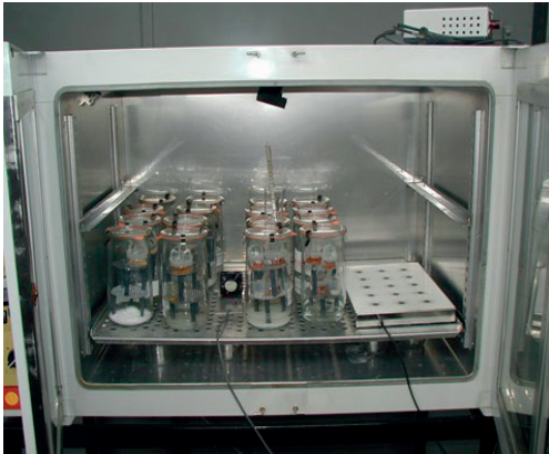
Figure 1. Temperature controlled cabinet HERAEUS type B 5090E with sorbostats
