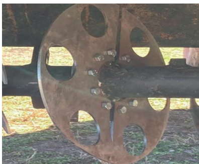
Figure 5. Disk with a horizontal axis of rotation and the horizontal displacement mounted on tractor
