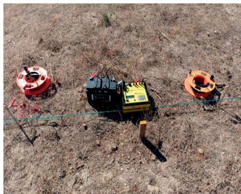
Figure 9. Field data acquisition using the Vertical Electrical Sounding (VES) method (McNeill, 1990)
