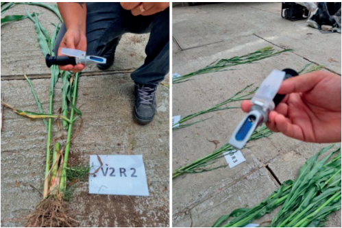
Figure 3. Determination of the sugar content in the stem by the refractometer method
