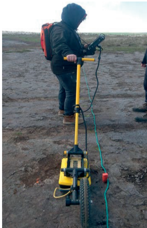
Figure 7. GPR data acquisition using the 100 MHz and 500 MHz antennas
