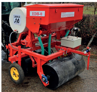
Figure 2. Mobile equipment for in-situ soil bioremediation - experimental model
