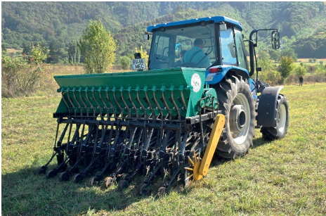
Figure 1. Experimental model of overseeding machine for degraded grasslands
