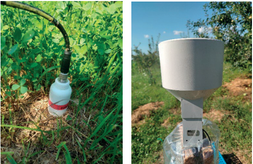
Figure 2. Soil moisture sensor and rain gauge
