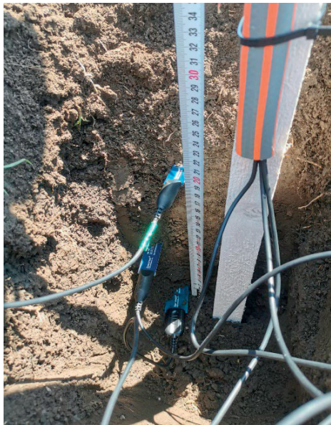
Figure 3. WatchDog 1000 Micro Weather Field Station with moisture sensor
