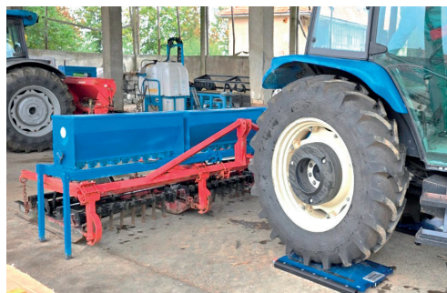
Figure 2. Aspects of the weighing process for the grassland planer experimental model coupled with the fertilization equipment
