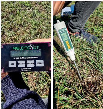
Figure 5. Field measurements of the main physical soil properties: penetration resistance and soil moisture content
