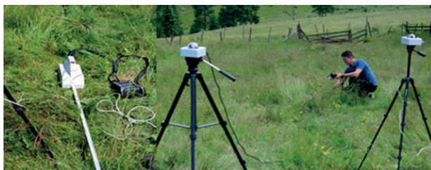
Photo 2. Measurements performed with the Sunscan Canopy Analysis System and the PAR sensors.
