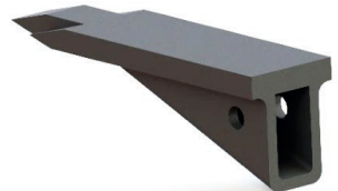
Figure 4. 3D geometric model of the chisel-type active organ variant V3 - cast in cast iron EN-GJMW-350-4
