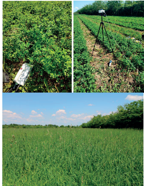
Figure 3. Delta-T Devices SunScan Analysis System deployed in the alfalfa canopy and the orchard grass field
