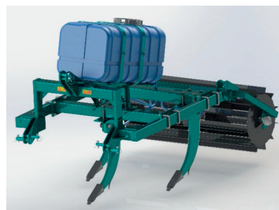
Figure 1. 3D geometric model made in SolidWorks of the innovative technical equipment for the processing and inoculation of a biofertilizer in the arable substrate
