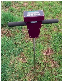
Figure 1. Soil resistance meter
