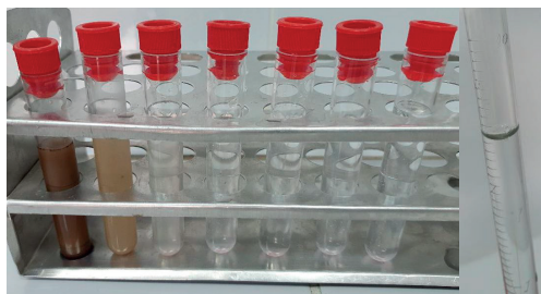
Figure 1. Preparation of decimal dilutions 10^{-1} \dots 10^{-7}
