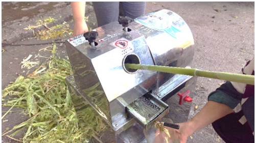
Figure 6. Electric roller press for extracting sweet juice
