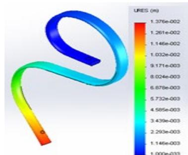
Figure 26. MS6 Model - The resulting relative displacement field in the structure (m)
