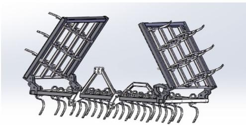
Figure 12. Device with active parts, transport position
