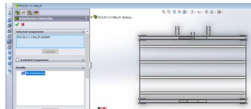
Figure 15. Central frame - interferences calculation
