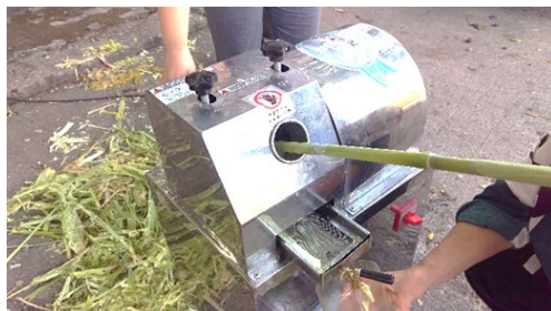
Figure 6. Electric roller press for extracting sweet juice
