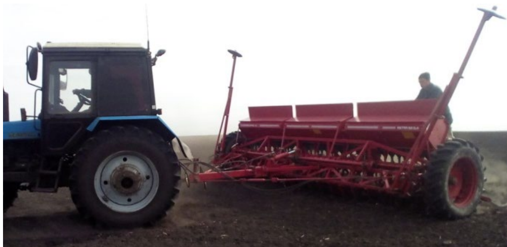
Figure 3 - General view of the seeder with experimental reel seeders
