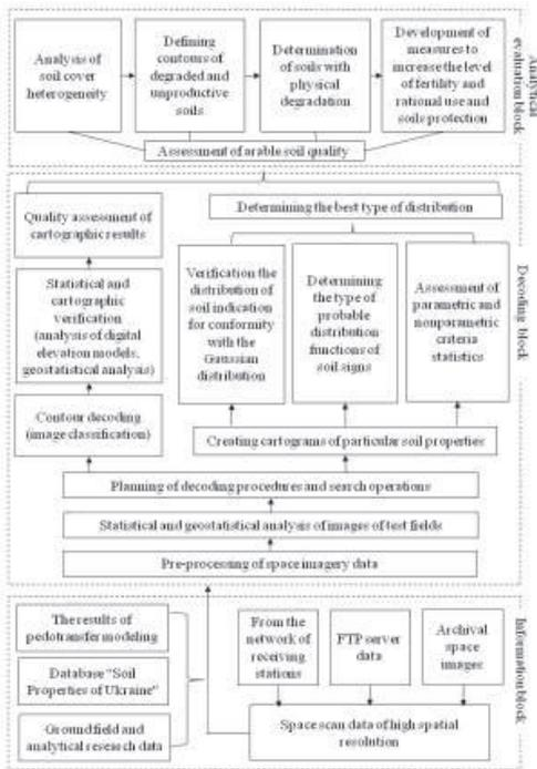
Figure 1. System of cartographic-analytical determination of degraded soils on the basis of space scanning data
