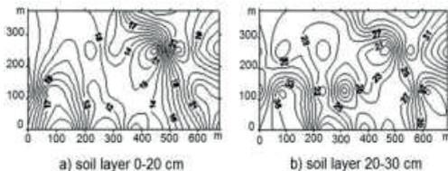
Figure 4. Two-dimensional models of soil penetration resistance distribution (Medvedev, 2009)
