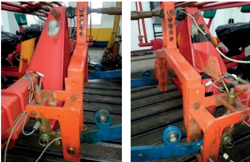
Figure 2. Tensometric frame for measuring tensile strength
