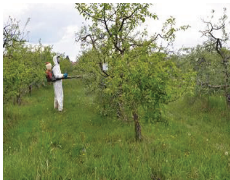
Figure 1. Field treatment with mist blower Solo 423 atomizer suitable for fungicide treatments in orchards
