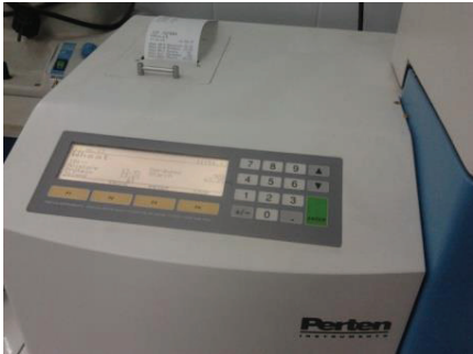
Figure 1. NIR Inframatic 9200 Product Instalab-Analyzer (Yield Quality Laboratory of Crops Sciences Department)
