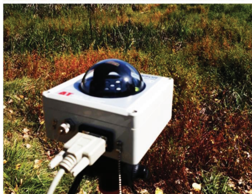
Figure 2. Instrumentation used for in situ monitoring of evapotranspiration at riparian grassland level in Poeni, Teleorman County (beam fraction sensor for PAR monitoring; digital anemometers; microclimate multiparameters; temperature sensors; soil moisture sensors)
