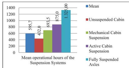
Figure 8. Chart showing the mean operational hours of the agricultural tractors surveyed, categorised by suspension systems
