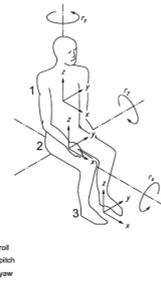
Figure 2. Diagram showing the  $x$ ,  $y$ ,  $z$  Axis Orientation, (ISO, 1997)
