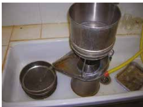
Figure 7. Apparatus of Fenwick for cysts extraction
