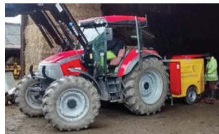
Figure 5. Tractor under test using a Fromet dynamometer
