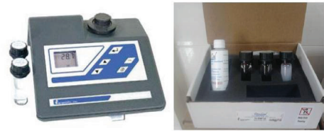
Figure 3. Turbidimeter Device (HF Micro 1000) and calibration kits
