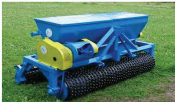
Figure 1. MSPFP-2.0 meadows forage sowing Machine
