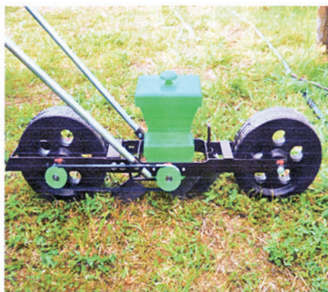
Figure 2. Small seed sowing machine in one row with mechanical distribution
