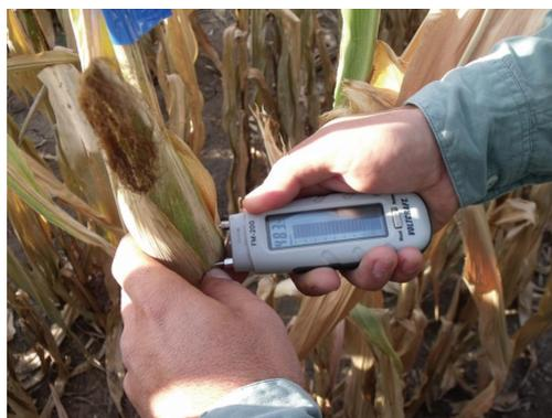
Figure 2. Measuring grain moisture with Voltcraft FM-200 Humidity meter, through the husks
