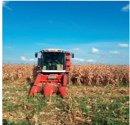
Figure 1. The BAURAL SP2100 harvester for experimental plots, on two rows
