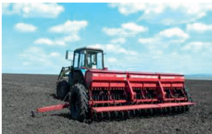
Figure 2. A seeder with combined coulters on the fields of Antonovo farm
