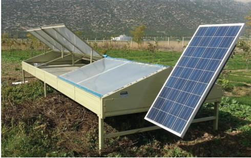
Figure 1. The experimental solar tunnel dryer
